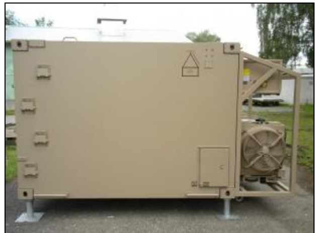
Outside view of 'Zagil' Shelter with power generator and air condition unit
