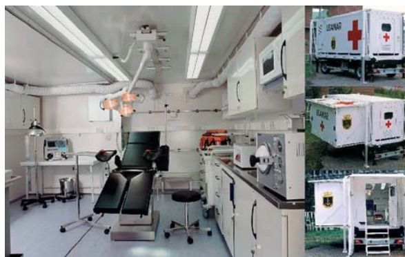
Fig. 1: Mobile Clinic or Rescue Station in a 1-side expandable shelter
